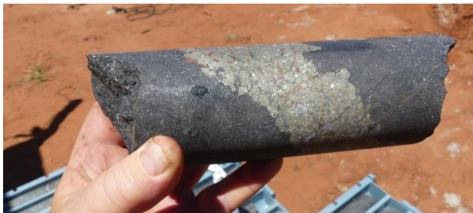
Photo 1: 21MHDD002 (275.4m) – massive magnetite skarn with disseminated scheelite and molybdenite mineralisation and bands of chalcopyrite.
