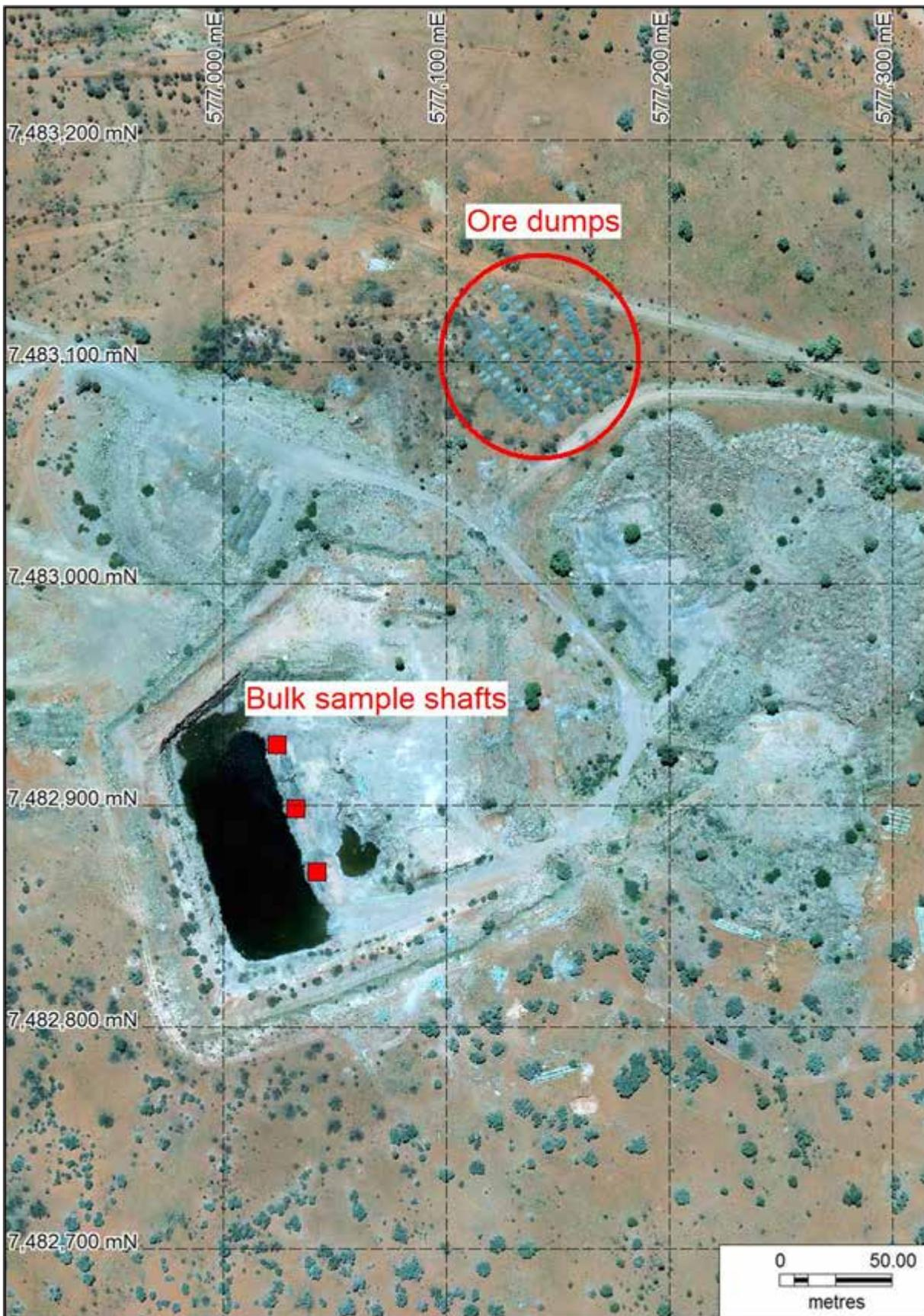
Figure 3: Detail of Molyhil mine site
